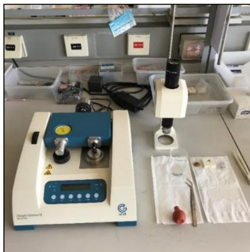
Figure 10. Gatan Dimple Grinder System.
