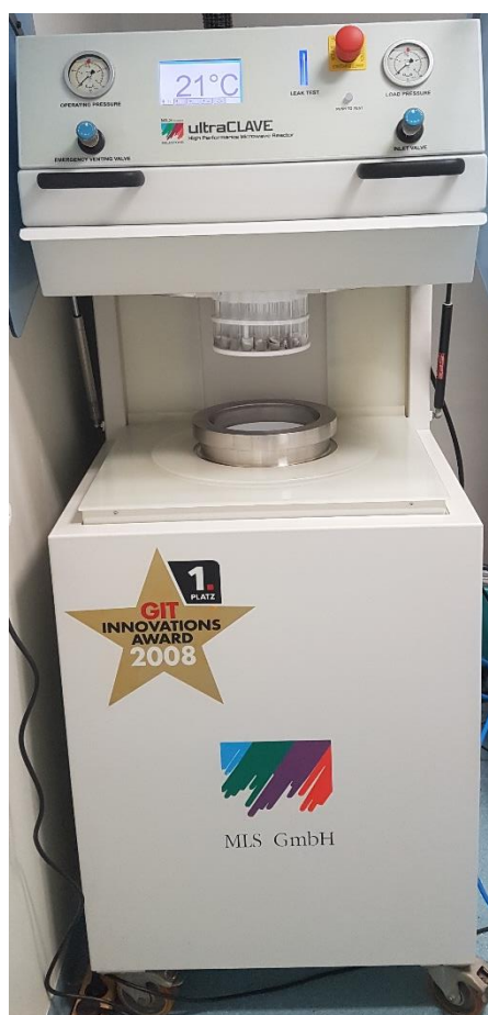
Slika 15. Mikrovalni reaktor High Performance Microwave Reactor – UltraCLAVE .
