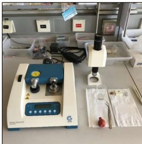
Figure 10. Gatan Dimple Grinder System.
