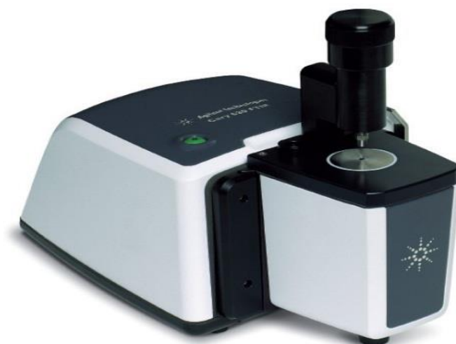
Slika 10. Cary 630 FTIR, Agilent Technologies
