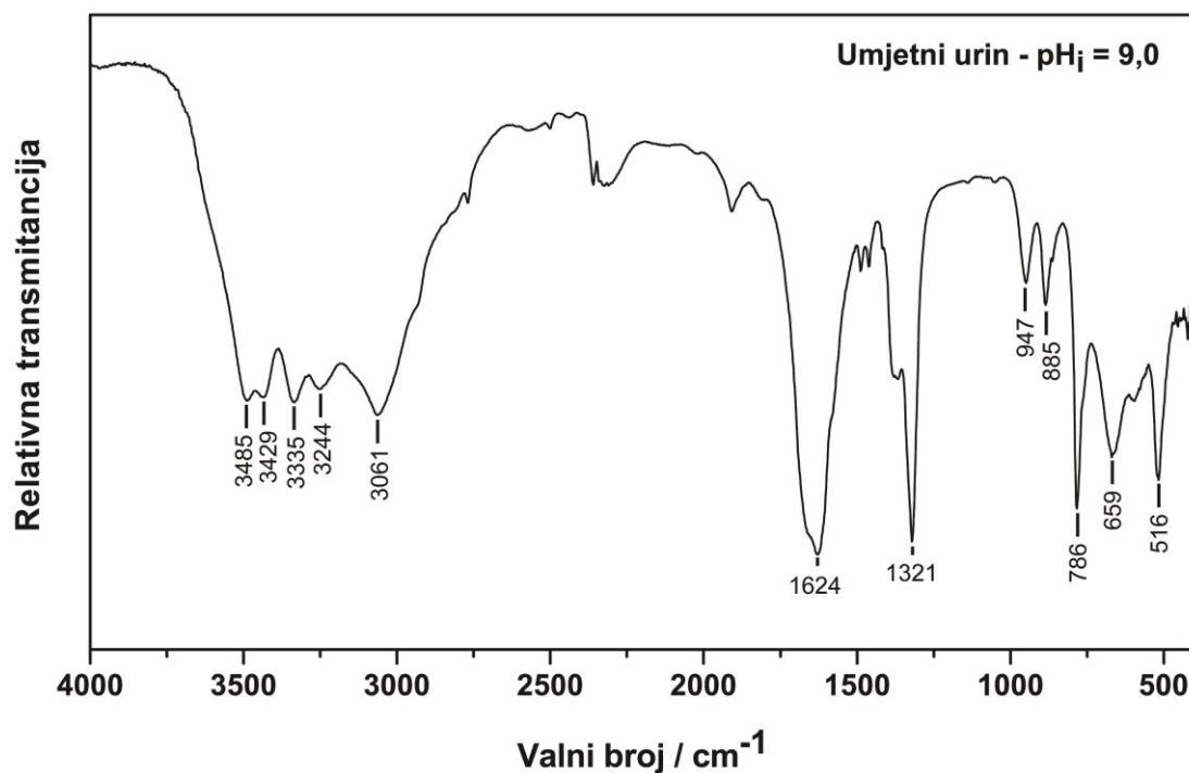
**Slika 31.** IR spektar uzorka istaloženog u sustavu umjetnog urina pri pH<sub>i</sub> = 9,0 (c<sub>i</sub>(Ca<sup>2+</sup>) = 7,5 mmol dm<sup>-3</sup> i c<sub>i</sub>(C<sub>2</sub>O<sub>4</sub><sup>2-</sup>) = 6,0 mmol dm<sup>-3</sup>)
