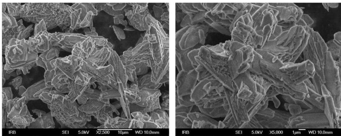
**Slika 34.** SEM snimke promatranog sustava istaloženog u sustavu umjetnog urina pri  $\text{pH}_i = 9,0$  ( $c_i(\text{Ca}^{2+}) = 7,5 \text{ mmol dm}^{-3}$  i  $c_i(\text{C}_2\text{O}_4^{2-}) = 6,0 \text{ mmol dm}^{-3}$ )
