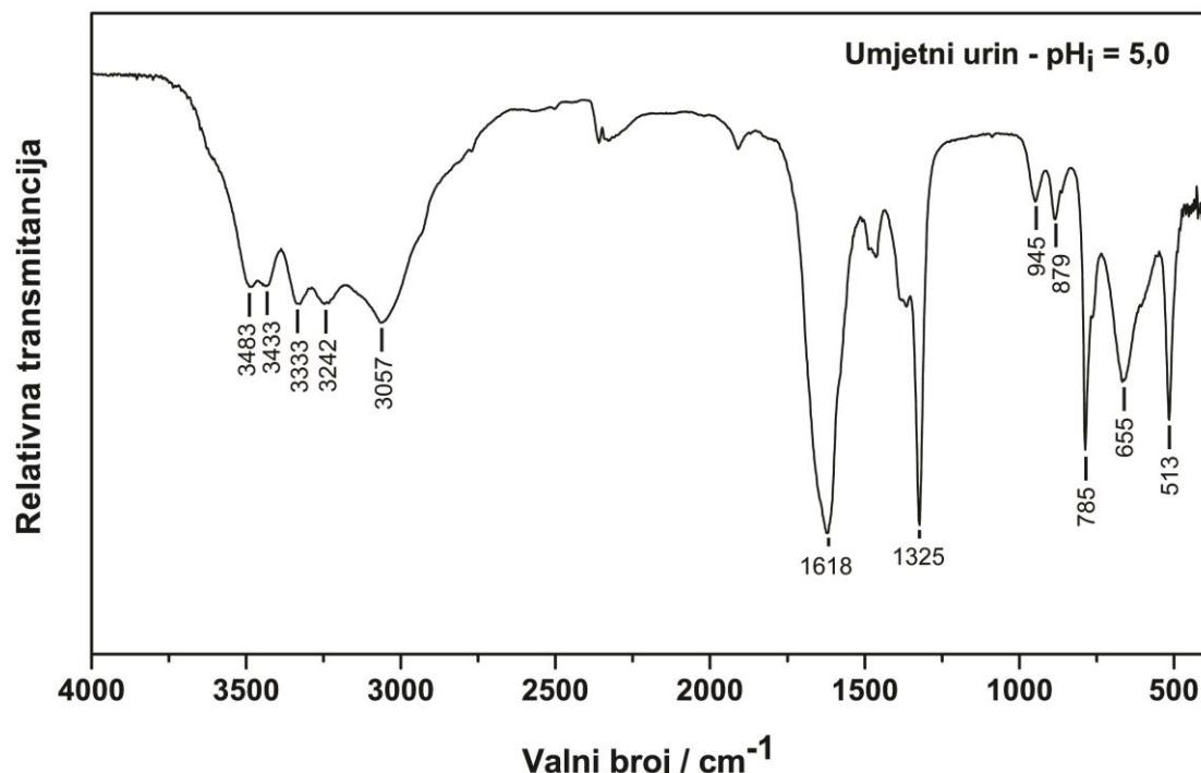
**Slika 26.** IR spektar uzorka istaloženog u sustavu umjetnog urina pri  $\text{pH}_i = 5,0$  ( $c_i(\text{Ca}^{2+}) = 7,5 \text{ mmol dm}^{-3}$  i  $c_i(\text{C}_2\text{O}_4^{2-}) = 6,0 \text{ mmol dm}^{-3}$ )
