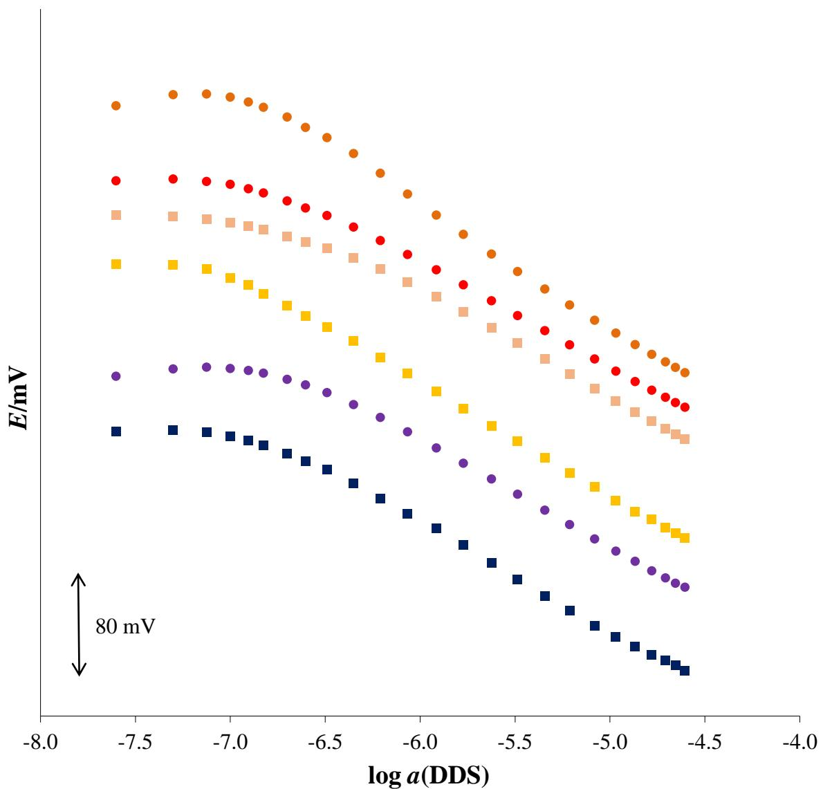
**Slika 21.** Odzivne karakteristike TODA-TPB senzora na DDS ( $c = 5 \cdot 10^{-5} \text{ M}$ ) u vodi (bez pauze i s pauzom) i  $0.01 \text{ M} \text{Na}_2\text{SO}_4$  (■ 3 M  $\text{NaCl}$  u vodi bez pauze; □ 3 M  $\text{NaCl}$  u vodi s pauzom; ■ 3 M  $\text{NaCl}$  u  $\text{Na}_2\text{SO}_4$ ; ● 0.5 M  $\text{NaCl}$  u vodi bez pauze; ● 0.5 M  $\text{NaCl}$  u vodi s pauzom; ● 0.5 M  $\text{NaCl}$  u  $\text{Na}_2\text{SO}_4$ ).
