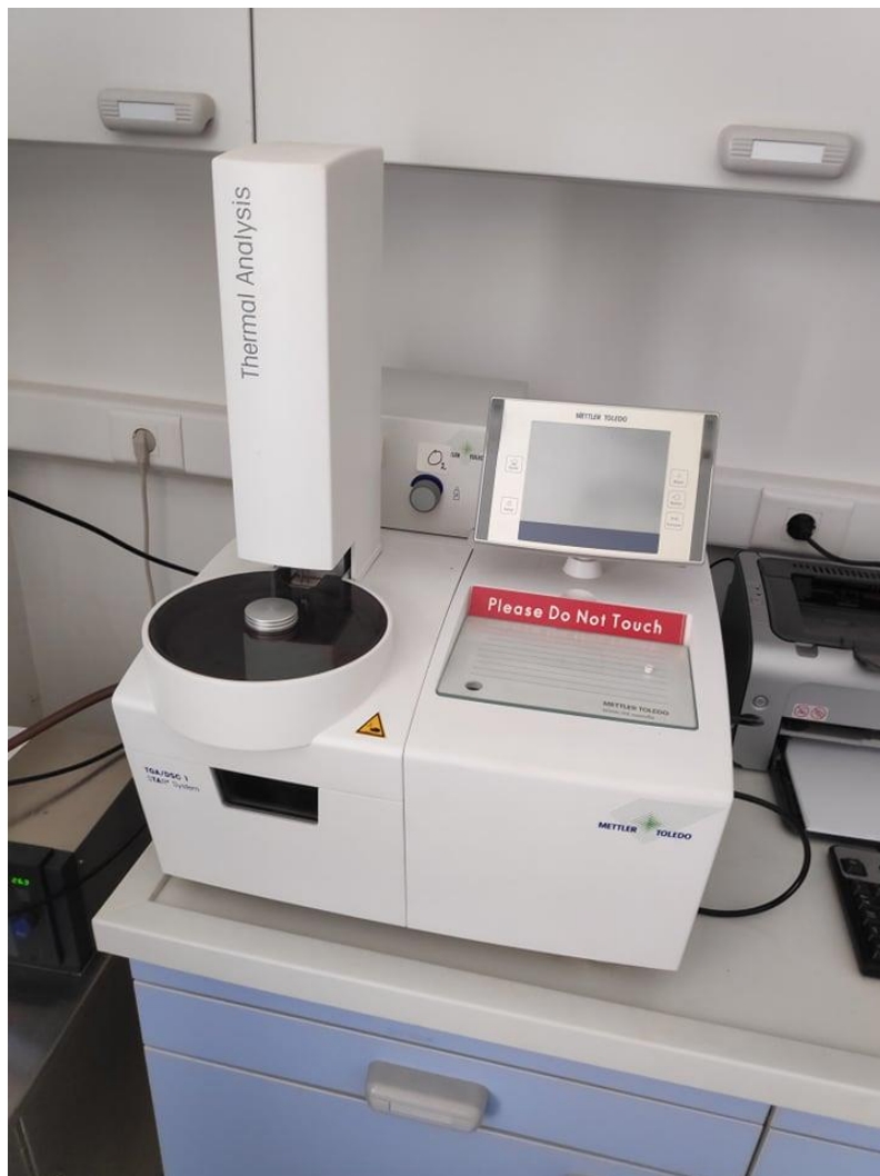
Slika 10. TGA/DSC 1, Mettler Toledo.
