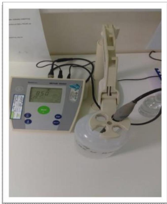
**Slika 9.** pH metar, Mettler Toledo.
