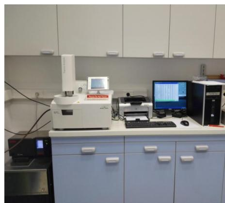
*Slika 12. Mettler-Toledo TGA/DSC model 1*
