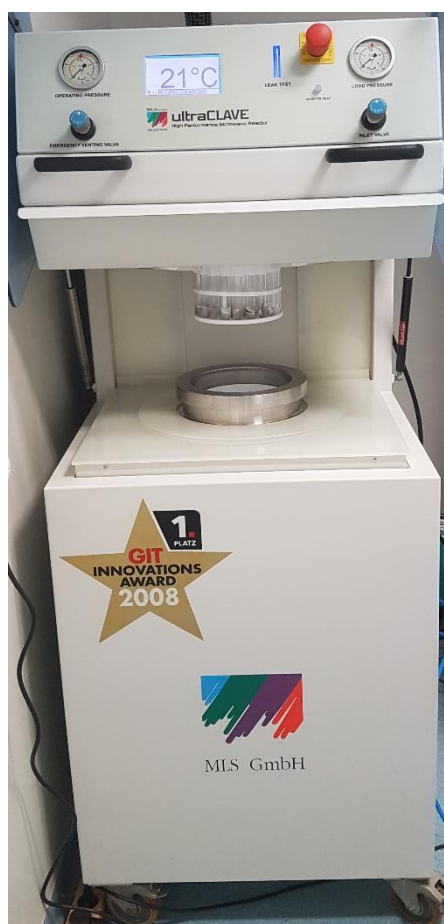
Slika 15. Mikrovalni reaktor High Performance Microwave Reactor – UltraCLAVE .
