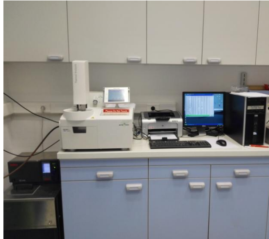
Slika 15. Mettler-Toledo TGA-DSC model 1
