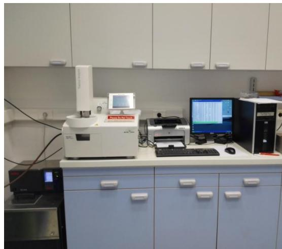
*Slika 15. Mettler-Toledo TGA-DSC model 1*
