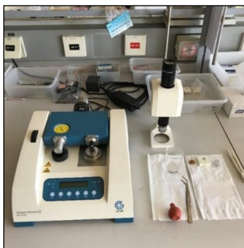
Figure 10. Gatan Dimple Grinder System.
