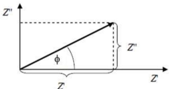
$$\begin{aligned} Z^2 &= Z'^2 + Z''^2 \\ |Z| &= \sqrt{Z'^2 + Z''^2} \\ \tan \varphi &= \frac{Z''}{Z'} \rightarrow \varphi = \tan^{-1} \frac{Z''}{Z'} \end{aligned}$$
