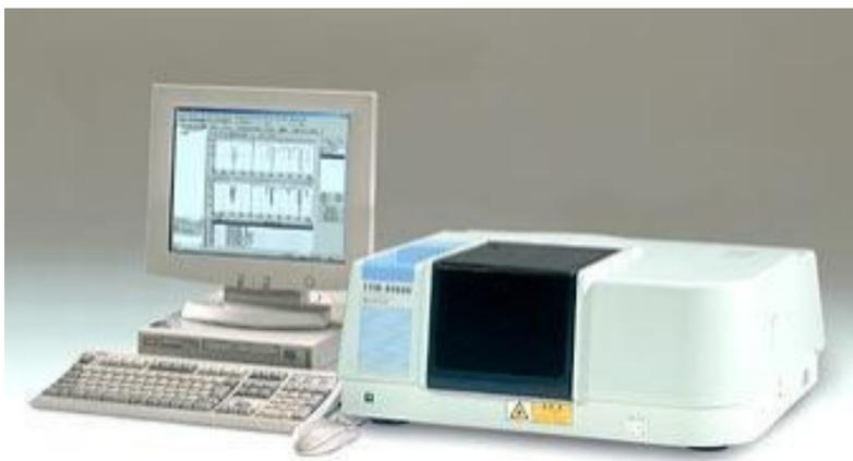
Slika 20. Spektrometar SHIMADZU FTIR-8400S. (izvor: <https://speciation.net/Database/Instruments/Shimadzu-Europe/FTIR8400S-;i1306>)
