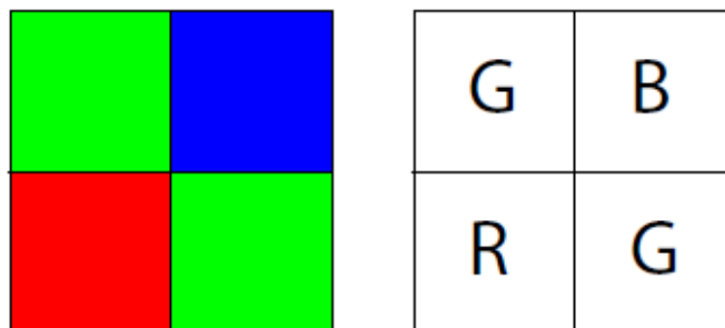
Slika 6. Bayerov raspored filtera
