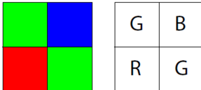
Slika 6. Bayerov raspored filtera
